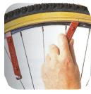
Insert the 2nd tyre lever under the tyre a few spokes from the 1st and slide it around lifting the tyre off the rim.
